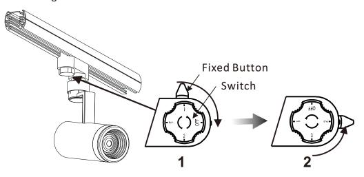
3. Select the phase and power you need. Connect the fixture to power and adjust the direction of light you need. Adjust the beam angle until appropriate.
